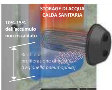
STRAIGHT HEAT EXCHANGER: between 10% - 15% of storage volume is not heated with relevant thermal inefficiencies and risk of Legionellosis bacterias diffusion.
