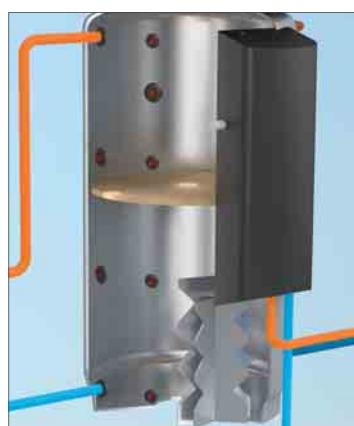
Performances are optimized thanks to the "Labyrinth Spreader" (Cordivari Patent). Its spread shape allows a perfect stratification of the water that returns back from the plate exchange to the tank. Heating installation efficiency is guaranteed.
