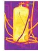
**Series of thermographs that illustrate the efficiency of the Cordivari patent through the perfect thermal stratification**
