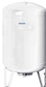
The preload value of the expansion vessel will be 0,3-0,5 bar less than pressure P<sub>i</sub>.
