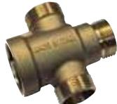
Auto-operated thermostatic switch valve, calibrated at 45°C. It can easily integrate solar thermal systems for DHW production with a boiler.
