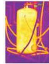
**Series of thermographs that illustrate the efficiency of the Cordivari patent through the perfect thermal stratification**
